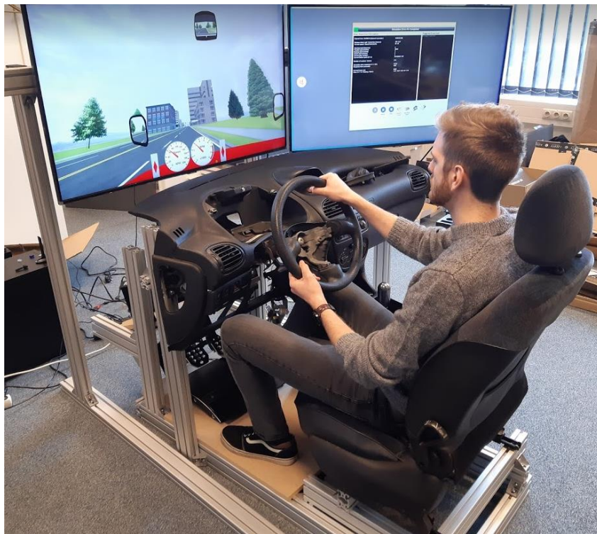
Figure 6: DSS Car simulator, using OEM Peugeot 206 parts
