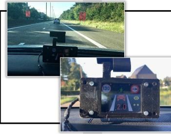
DSS tests their prototype real-time intervention technology in a vehicle. This provides better insight into the placement, readability under different lighting conditions and comprehensibility. This way it becomes clear where there is room for improvement.
