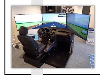
DSS developed a custommade driving simulator system based on parts of a Peugeot 206. In this way, the reality is simulated as truthfully as possible and the i-DREAMS monitoring and intervention technology can be tested and optimised before being rolled out in field studies.
