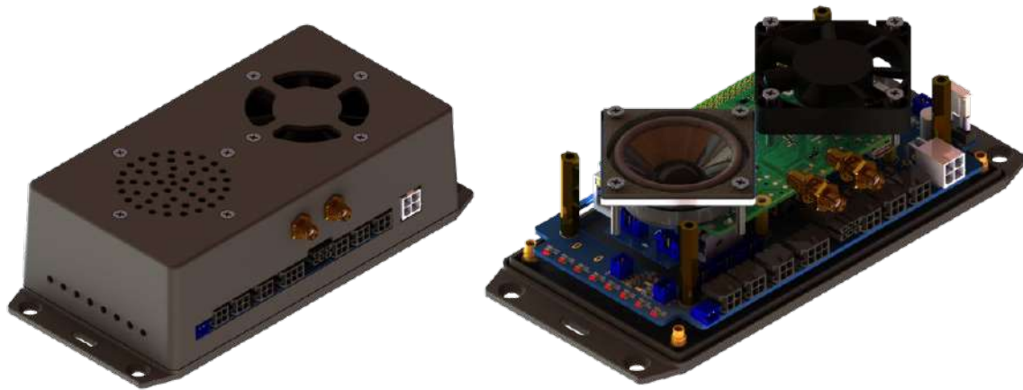
Figure 6: Final CardioGateway form-factor (external and internal views).
