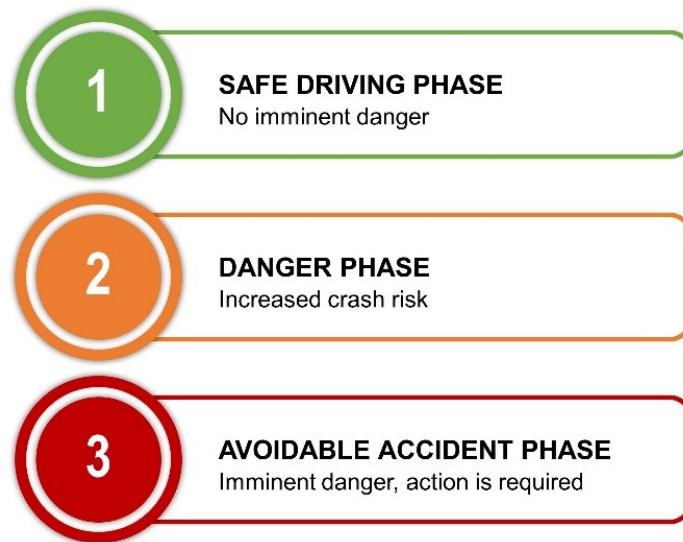
Figure 1: The three phases of the STZ
