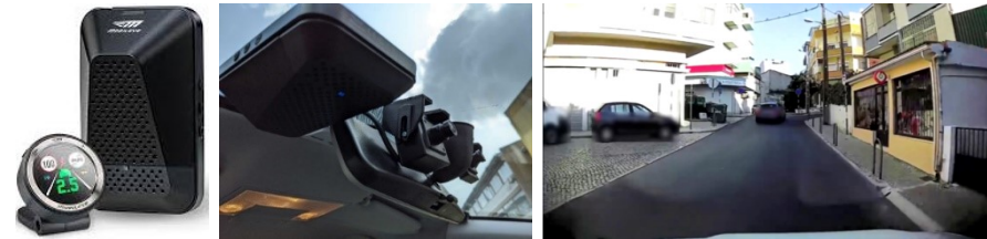
Figure 5: Mobileye, including eyewatch (image 1), Mobileye and dashcam fitted in a vehicle's windshield (image 2), blurring of license plates (image 3)
