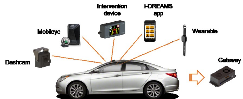
Figure 2: i-DREAMS suite of technologies for cars
